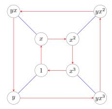
The red arrows represent multiplication by x from the left, and the blue edges represent multiplication by y; since  $y = y^{-1}$ , the blue edges are undirected. The dihedral group of order 8 can be also given by the following presentation:  $D_8 = \langle a, b | a^2 = b^2 = 1, (ab)^2 = (ba)^2 \rangle$ . In this case, Cay $(D_8, \{a, b\})$  is as follows:
